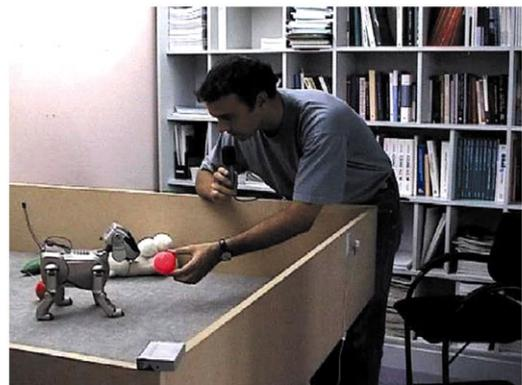
**Fig. 1.** The AIBO™ pet robot has been used in experiments to see how language-like communication in robots might be bootstrapped by interaction with a human mediator. Reproduced with permission from Ref. [12].
