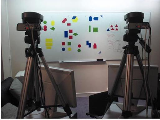
**Fig. 2.** The 'Talking Heads' experiment featured two pan-tilted cameras oriented towards a white board on which geometric figures were pasted. Agents used these cameras to play lexical games drawing attention to a chosen figure, which is the 'topic' of that game.
