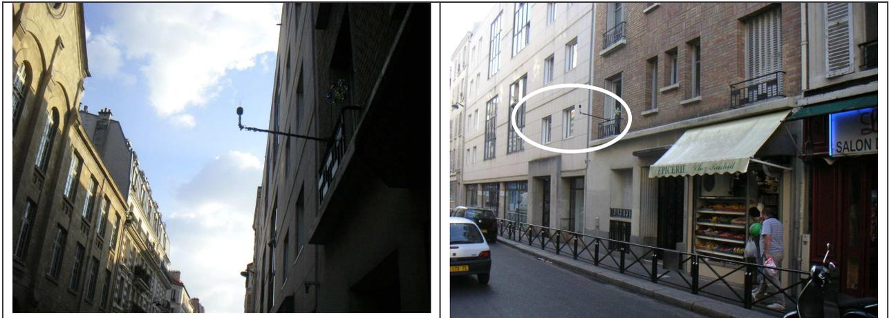
Figure 3 : microphone placed 2 meters away from balconies and 4 meters high from the street. The microphone is connected to a computer that calculates in real time features such as  $L_{Aeq}$ , octave bands and sound source identification.
