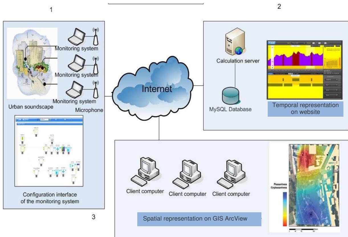
Figure 2 : synopsis of FDAI system. It consists of three main modules interconnected through IP. Module 1 sets up the monitoring systems, module 2 deals with the conditioning of the data measured on a server and provides temporal representation through the website; module 3 provides spatial representation through animated maps on GIS (Geographic Information System).
