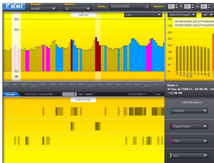
Figure 4 : Temporal representation of soundscape features through Web interface. This screenshot represents on top the evolution of the  $L_{Aeq}$  measured on one location. The colours are the projections of the most prominent identified sources mentioned on the bottom (Voiture means car, Cyclomoteur means moped, Voix means voice). On top right, octave-band energy of a selected part of the  $L_{Aeq}$  curve is calculated.
