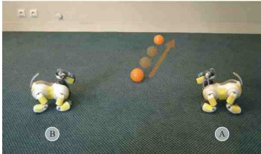
Figure 1: Agents embodied in physical robots. The speaker (in robot A ) and the hearer (in robot B ) together observe ball movement events and then play a language game to describe the scene to each other.
