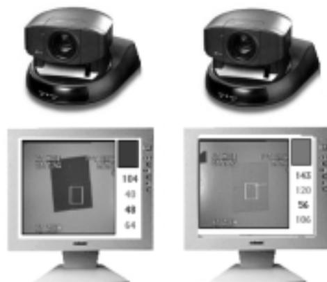
to be speaker or hearer. Agents are capable of segmenting the image perceived through the camera into objects and of collecting various sensory data about each object, such as the color (decomposed in RGB channels), average gray-scale or position. The set of objects and their data constitute a *context*. The speaker chooses one object from this context, further called the *topic*. The other objects form the *background*. The speaker then gives a linguistic hint to the hearer.
