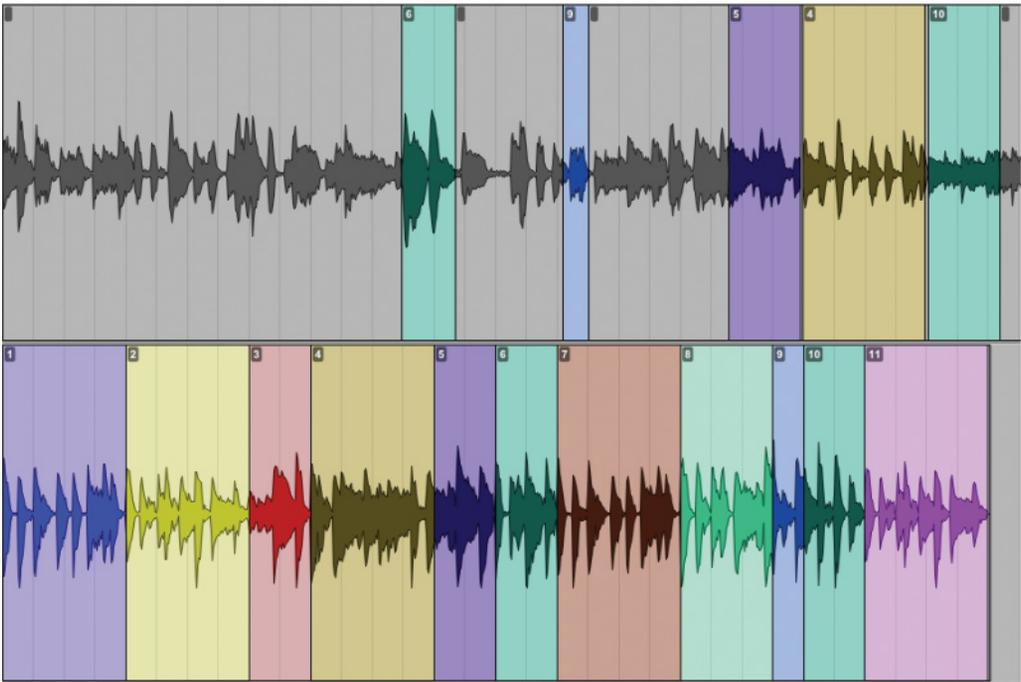
Fig. 5. Groove-preserving concatenative synthesis to generate a convincing bossa nova accompaniment of *Ode to Joy* (extract). Segments of the source audio file (top) are reused, modified, transposed, and stretched to generate the target (bottom).
