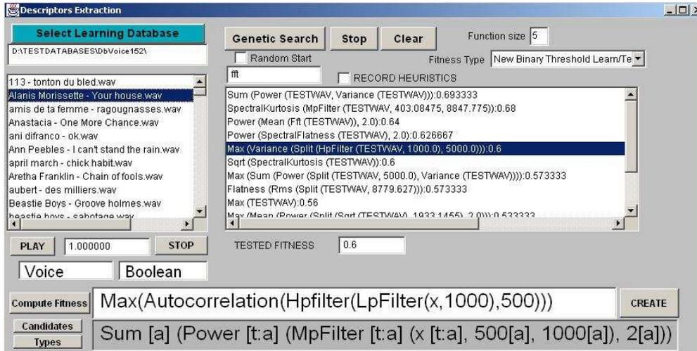
Figure 4. The EDS system finds automatically signal processing functions that extract high-level descriptors from acoustic signals. On the left part, a database of songs for which human perceptive tests have been performed is used to evaluate functions. EDS contains heuristics and rewriting rules to guide its search and simplify expressions. Here the expression in the text field is simplified, and its type is inferred (below).
