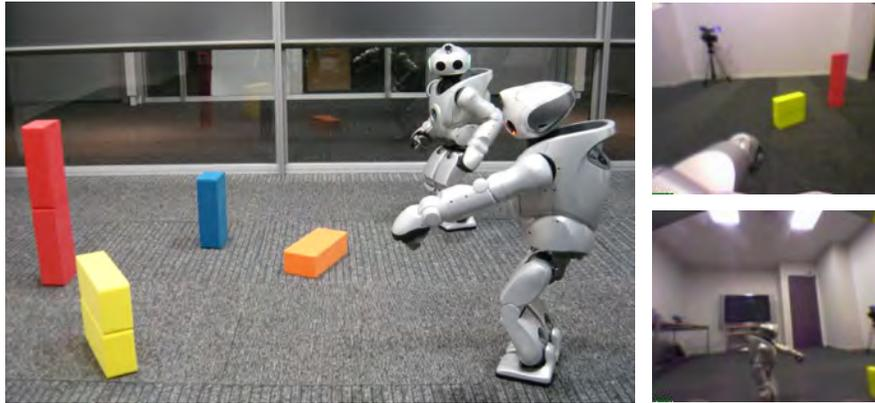
**Fig. 5.6** Demonstration of a Sony humanoid robot drawing the attention of the other robot to an object in the shared environment by pointing at it. The images at the right show the scene as seen through the camera of the pointer (top) and the robot observing the pointing (bottom). However, please note that the robots are not able to detect pointing gestures using their built-in cameras. Instead, they directly transmit  $x, y$  coordinates of the object pointed at.
