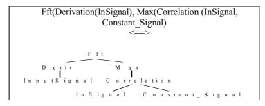
Fig. 3. Tree representation of a signal processing function
