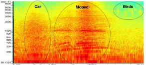
Figure 1. Sonogram of a sequence containing a car, a moped and birds.
