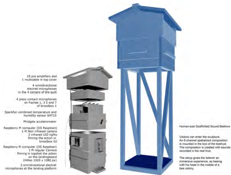
Fig. 5. Left: Diagram of the instrumented Sound Beehive, Right: the Scaffolding Sound Beehive Sculpture
